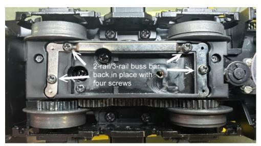
With the nubs in their new position, use the four screws to re-install the buss bar and then re-attach the center rail rollers.
