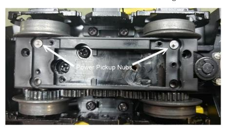
Underneath the metal bus bar are two power pickup nubs. On this truck, they are in the bottom position (Sorry that the photo does not show this exactly – the nubs can be moved and I was already playing around with that.) The nubs just sit in a hole in the plastic. You can grab them with needle nose pliers and just lift them out.
