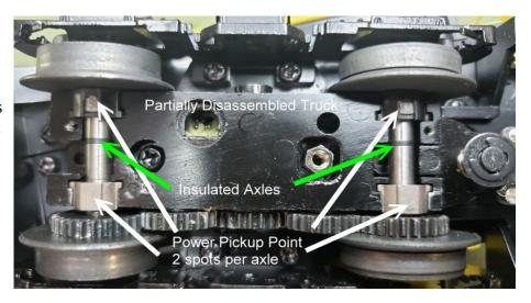
traction tire axle is useless. Since the traction tire insulates the wheel from the track, there is never any power at that pickup point.
