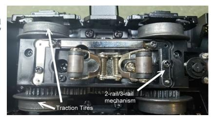
I removed the center rail rollers and the 4 screws holding the buss bar. Here is a photo what I saw.
