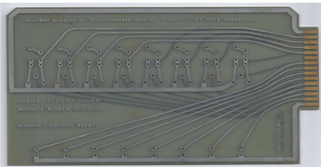
The above two photos show both sides of the double sided relay relay card which I chose to name the CMU-JCH-#02 card with a suffix of A for the component side and B for the solder side as shown.
